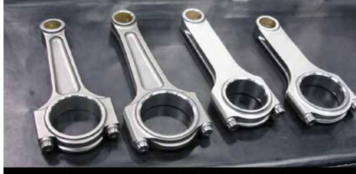
Connecting rods come in various styles and lengths. Choosing the one that's "right" for a given application depends more on strength, loading and RPM than rod ratio.
